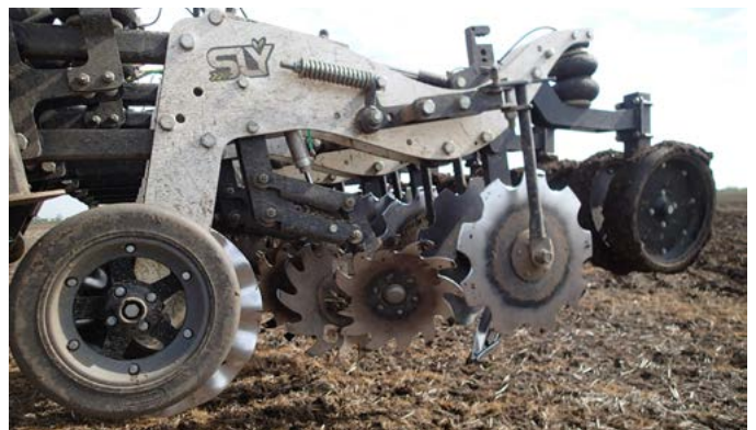
Figure 28. Specialised strip-till cultivation units prepare ground for later drilling
