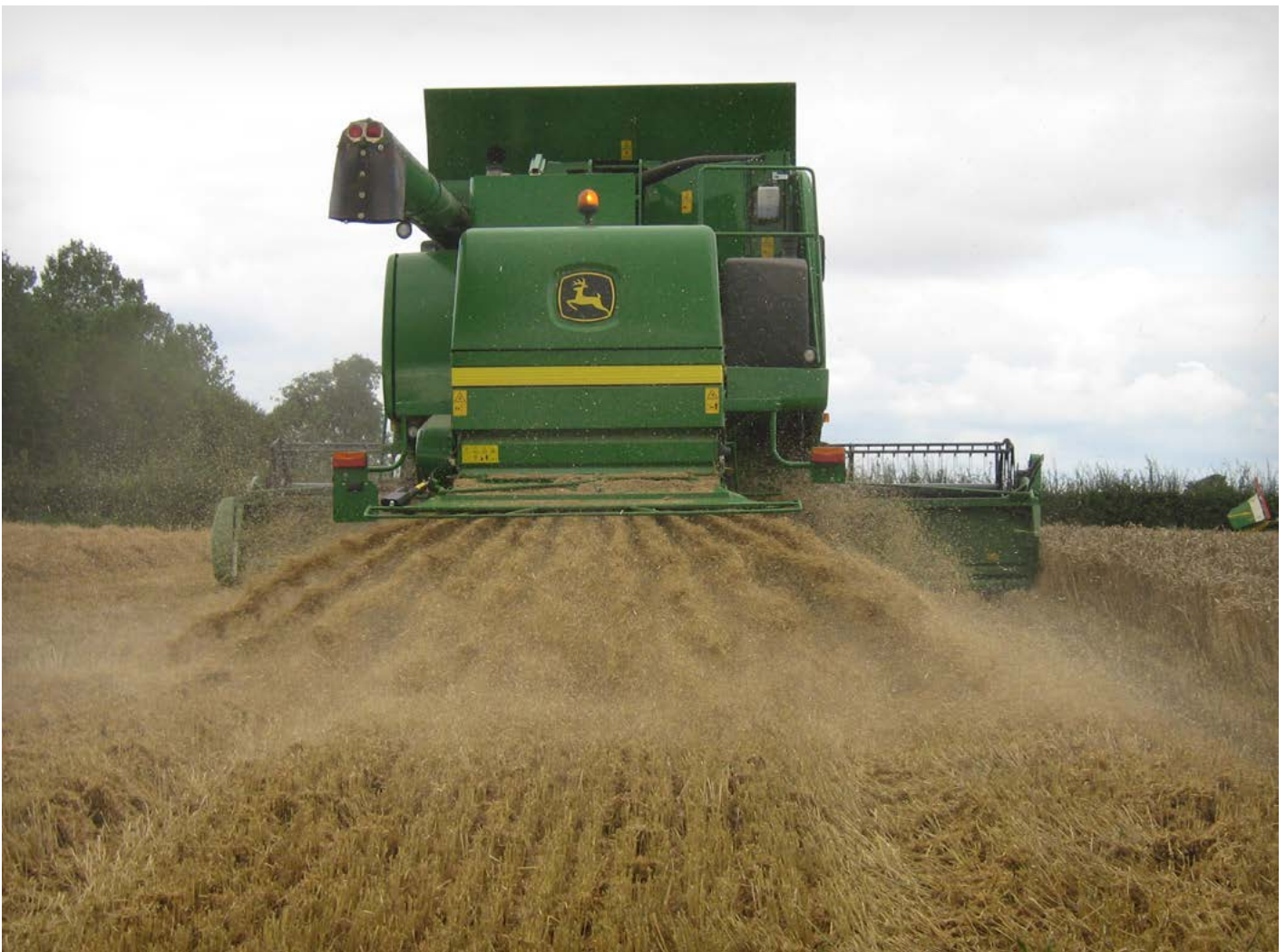
Figure 2. When straw is chopped, aim for an even spread to the full header width
