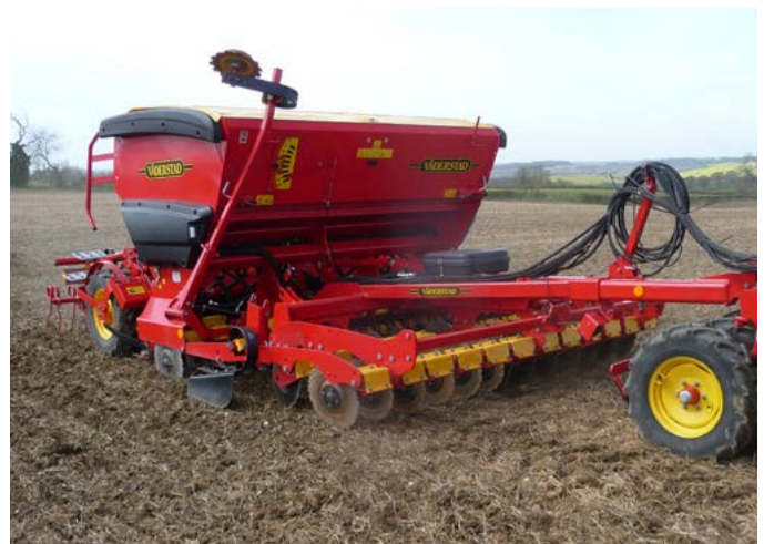
Figure 31. Combined structuring and drilling (top) and cultivator drill used as a direct drill with cultivation elements raised clear of work (bottom)
