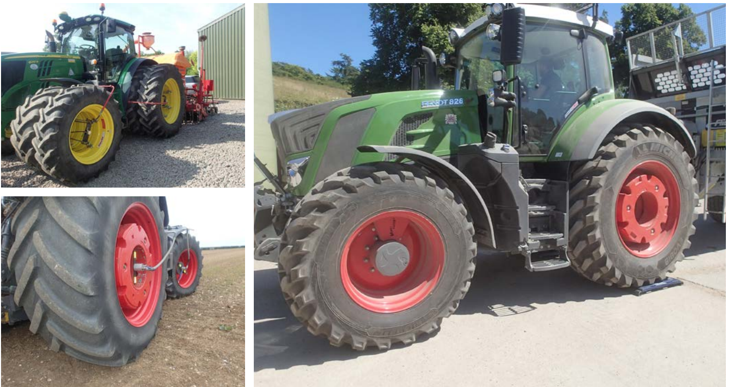
Figure 8. Retro-fit central tyre inflation system (CTIS) options (left, top and bottom) and original-fit, fully integrated CTIS (right)
