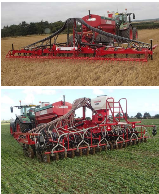
Figure 6. Cover crop established into a stubble with a relatively high-disturbance tine drill (top). Main crop drilled into a cover crop with a low-disturbance, disc-based drill (bottom). Both drilling modules can be mounted on the same leading hopper
