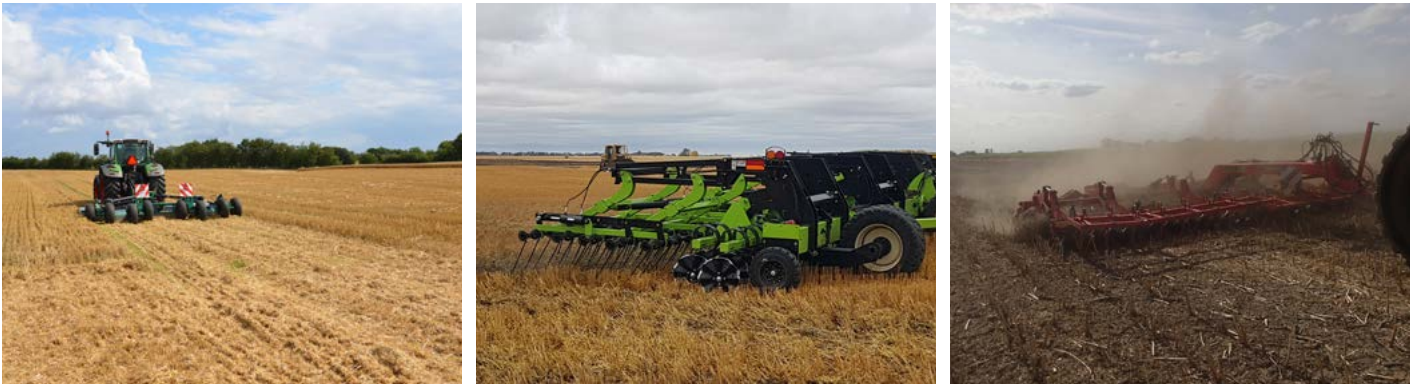
Figure 3. Residue management after harvest: stubble mulcher (left), straw rake (middle) and shallow cultivator (right)
