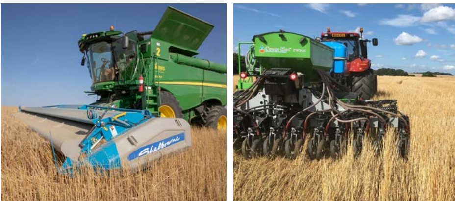
Figure 4. Long, anchored stubbles left by stripper heading (left) can be drilled with a suitable direct drill. Note: requires effective chaff spread
