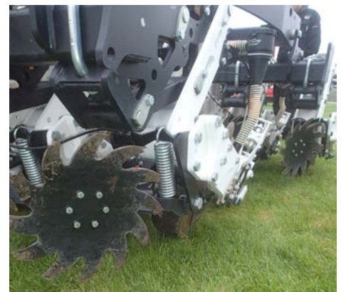
Figure 5. Example of residue managers fitted ahead of drill coulters
