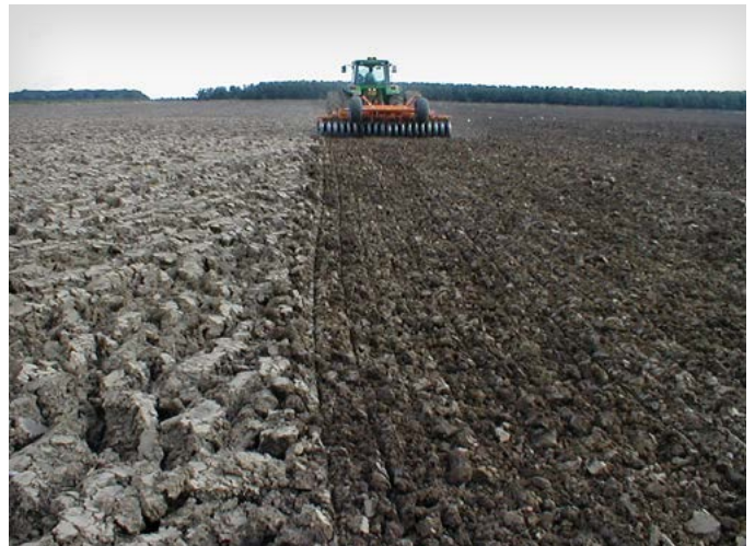
Figure 20. Pressing a ploughed field has many advantages
