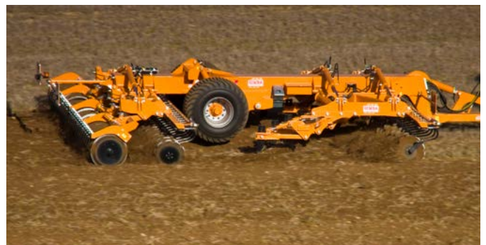
Figure 23. Typical high disturbance, deep non-inversion mixing action
