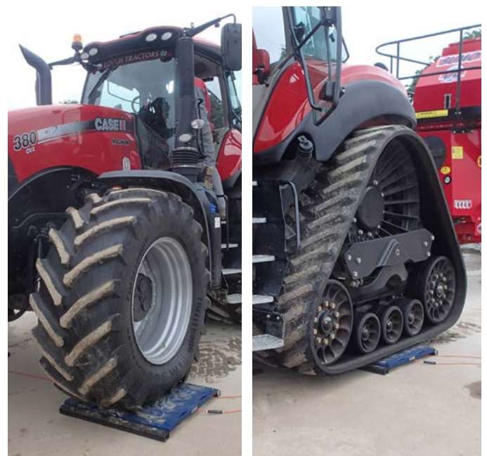
Figure 7: Use weigh cells to determine the maximum ballasted axle loadings for various operations. Once done, adjust tyre pressures accordingly. This is also important for the front tyres on half-tracked tractors, which can otherwise exert high pressures
