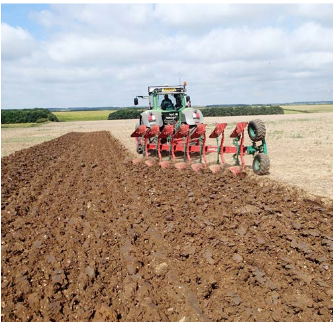
Figure 21. On-land ploughing to minimise furrow-base damage, compaction and to assist bout matching
